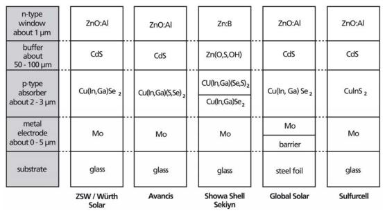
Figure 1. Structure of CIS Cells by leading manufacturers, Source: Fuhs (2009), p. 51
